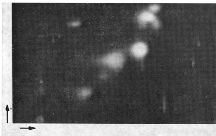
Fig. 2. Two-dimensional TLC of a 70% ethanol dorsal-skin extract from young larvae of Pachymedusa dacnicolor on a combination plate. The preparation and chromatography of this plate was as described in the text. The ethanol extract was prepared as outlined previously 1 , and 50 \mu l of sample was applied to the plate at the origin in the lower left corner. Arrows indicate the direction of migration.
